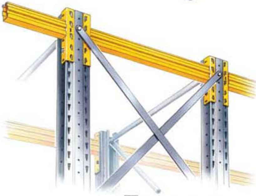
17 Detail of the bracing (at the top)
