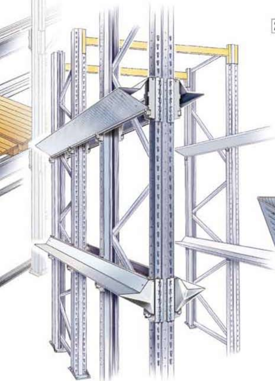
21 Double Sided DRIVE-IN guide rails located on single brackets
